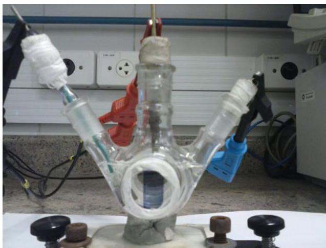
Figure 1. Three-electrode electrochemical cell with two quartz windows and \text{WO}_3 blue colored thin film inside the cell.
